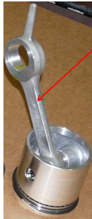
One-piece connecting rod
